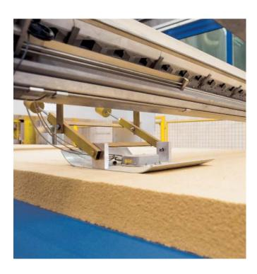
Habasit's proven anti-sticking belt ENB-12ERCH minimizes adhesion of panel chips and fibres and thus significantly improves product quality. The modified surface of the forming belt prevents residues on the belt and so ensures a longer service life.
